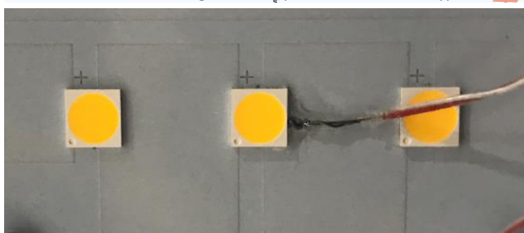
Figure 3. The recommended T_s point is located in the bottom of LUXEON 5050.
