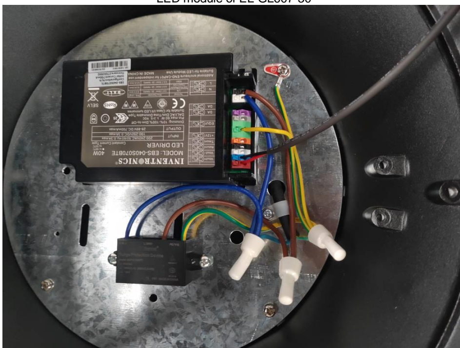
Internal construction of EL-GL607-30
