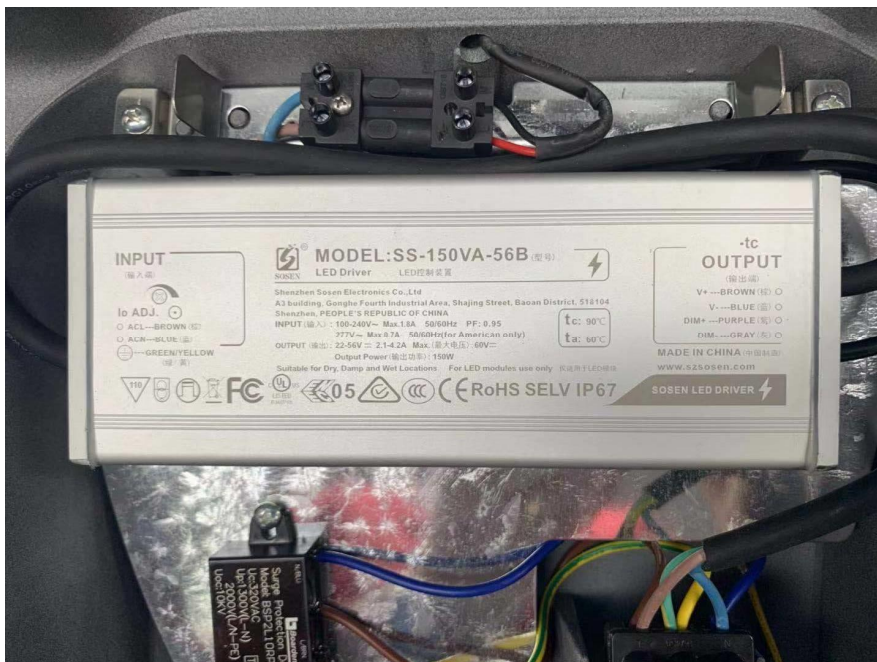
LED Driver of SS-150VA-56B
